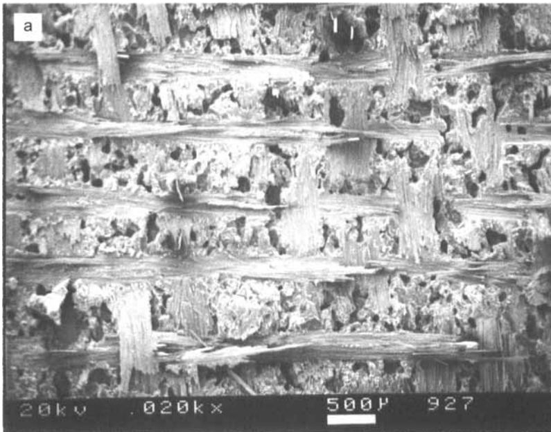
FIGURE 3 SEM photomicrographs of failure surfaces from wedge test specimens: (a) and (b) are side-A and side-B of the failure surfaces of samples that were thermally treated at 371°C for 3 hrs in air and then bonded; (c) and (d) are side-A and side-B of the failure surfaces of specimens that were bonded and thermally-treated at 371°C for 3 hrs in air.
